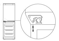
**13.** Carefully slide the fridge compartment door onto the top bearing pivot and close.
